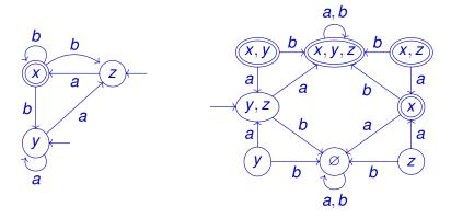
• new state space:  $2^X = \{V \mid V \subseteq \{x, y, z\}\}$
